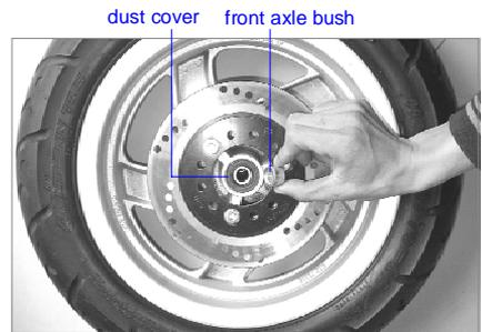
Turn bearing inner race to inspect sliding. Replace it with a new one in case of no sliding or damage or loosening of inner race.
